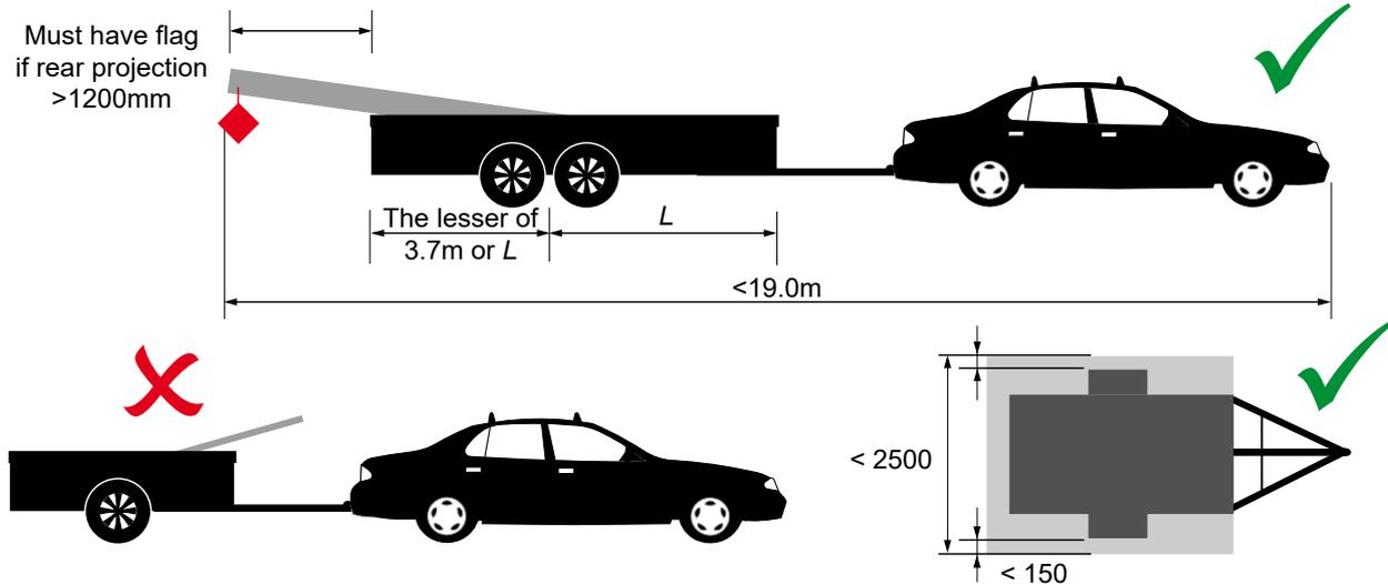
Towing a trailer does not change the amount of rear projection that is permitted on the tow vehicle.
