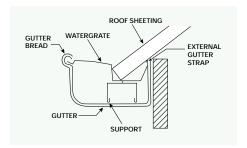
Support blocks are available from WaterGate® stockists. Position support blocks one metre apart install as shown above.
