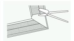
Insert further lengths, allowing a 25mm overlap. At corners, cut to 45° with tin snips and butt together.
