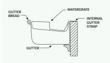
2. Lower WaterGate® until it sits on the internal gutter straps.
