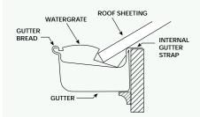
Wearing heavy gloves, compress the WaterGate® by hand, by pushing it against the back of the gutter.
