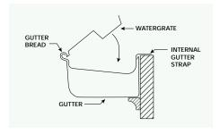
Insert the small 'v' shaped end of WaterGate® into the gutter's outer edge bead.
