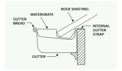
This will allow you to insert the outer 'v' shaped edge into the gutter's outer edge bead, clipping the WaterGate® securely in place.
