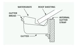
Position WaterGate® as shown so the flat edge slips up under the roof's edge and is supported beneath by the internal gutter straps.
